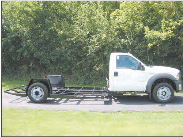
Galvanized Low Floor "Z" frame with axeless rear suspension
